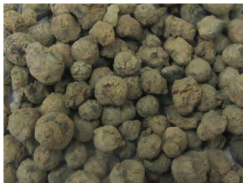
Figure 3: Sintered fly ash lightweight aggregate [15]
